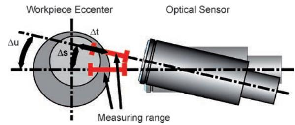
Fig. 3. Calibration of measuring system with an eccentric plate artefact.
