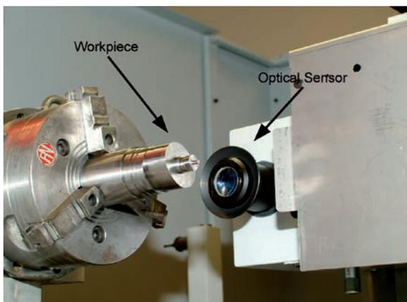
**Fig. 6.** Cylindrical grinding machine with integrated optical sensor and workpiece.
