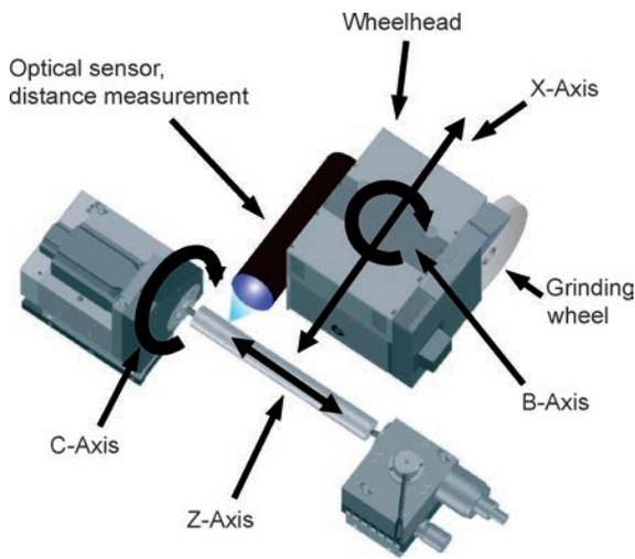
Fig. 1. Arrangement of the optical sensor on the wheel head in the grinding machine.
