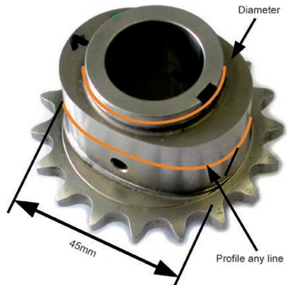
Fig. 5. Pump component, typical measuring tasks.
