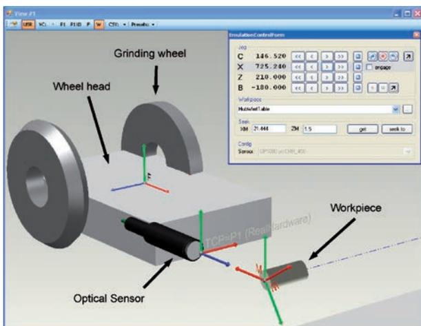
Fig. 2. Simulator of arrangements, coordinate transformations and tests.
