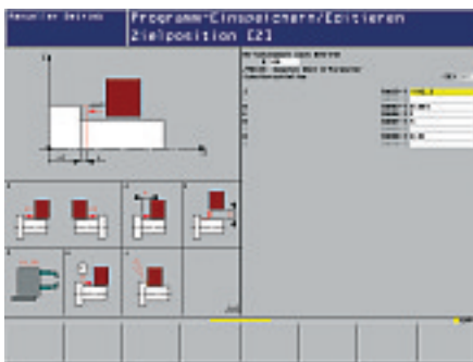
The form editor included in 'GrindPlusIT' makes set up and programming significantly easier for both grinding and dressing operations.
