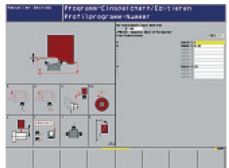
Below: Much easier: CAD drawings of workpieces needing to be ground can be easily (and instantly) imported as DXF files into 'GrindPlusIT' – making graphical programming using the graphics editor much quicker and easier.
