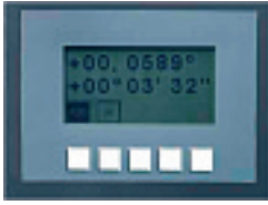
Top: As an optional feature, a swivel-angle display for the W spindle can be incorporated into the control panel.
