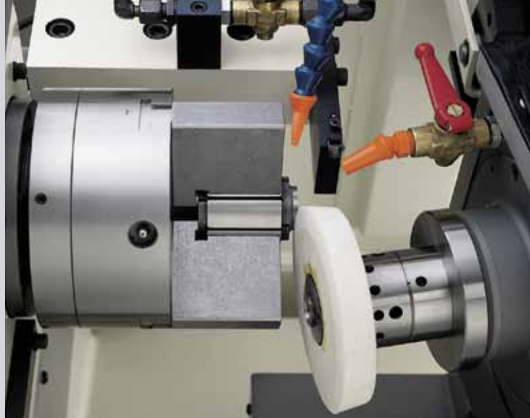
Typical example of external grinding
