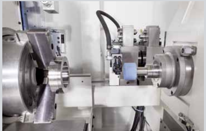
Working area with clamped work piece and grinding spindle
