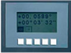
Top: As an optional feature, a swivel-angle display for the W spindle can be incorporated into the control panel.
